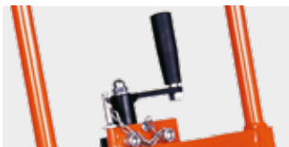
DEPTH CONTROL HAND WHEEL
