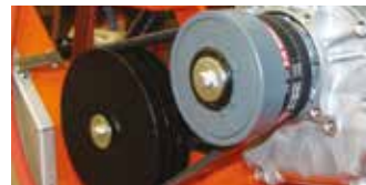
CENTRIFUGAL CLUTCH DEVICE
