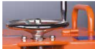
HANDWHEEL WITH ENDLESS SCREW DEPTH CONTROL SYSTEM
