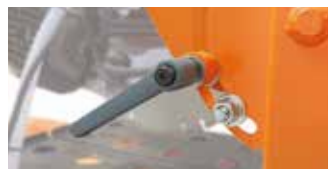
ADJUSTABLE CUTTING-DEPTH HANDLE
