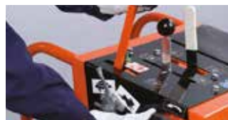
MANUALLY OR HYDRAULICALLY RAISE AND LOWER THE BLADE
