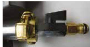
DUAL WATER-INLET AND DUST-COLLECTOR CONNECTOR
